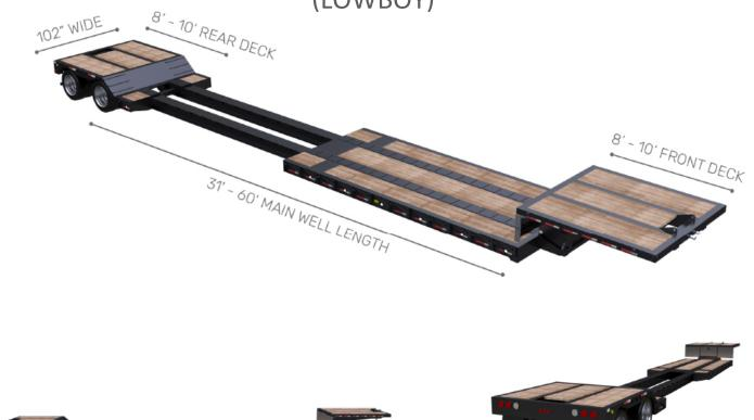
Extendable Double Drop trailers are utilized to transport oversized freight, both legally and through the use of permits and/or escorts. The primary difference between an Extendable Double Drop trailer and a standard Double Drop trailer is the ability of the Extendable trailer to extend/stretch out the well via two bars which allows for the transportation of longer commodities of up to 60' in length. Full tarping options are available as needed.
