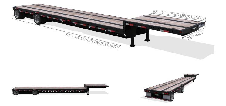
Step Deck trailers are primarily used to transport products that are too tall for a normal Flatbed trailer. There is an upper deck and a lower deck. The lower deck, called the well, allows for freight up to 120" high to be legally transported, while still providing the same loading/unloading capabilities of a standard Flatbed trailer. Specialized Low Pro Step Decks can manage freight that is up to approximately 126" to 128" in height.
