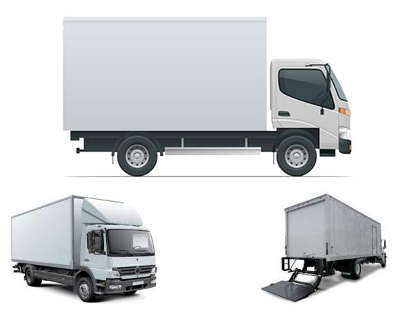
Similar to Dry Vans as they allow for dock-level loading/unloading and protect product from the elements. The main difference is in the capacity. A Straight Truck is typically 20' to 28' in length which is ideal for picking up or delivering to locations where space is limited. Many Straight Trucks are equipped with Tailgates that allow for ground-level access where no dock is available.
